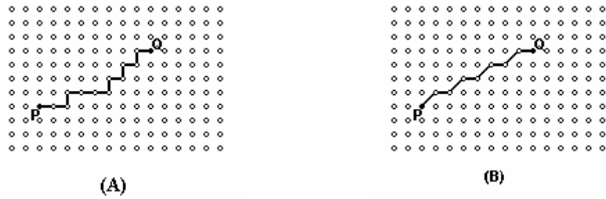
Figure 3.5 Discrete distance: (A) d_4(P, Q) (B) d_8(P, Q)
