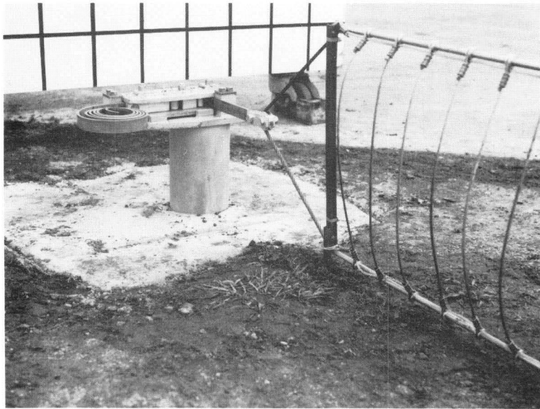
Figure 3, Metal Bender with 25,000 lb. Tape Attached to Net.
