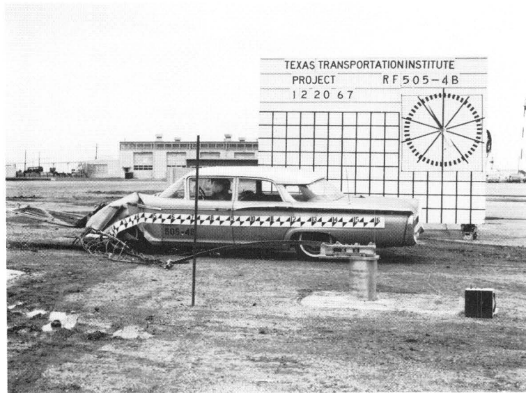
Figure 10, Vehicle and Left Metal Bender After Test 505-4B.
