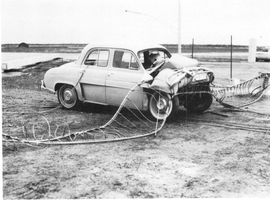
Figure 5, Vehicle and Dragnet after Test 505-4A.
