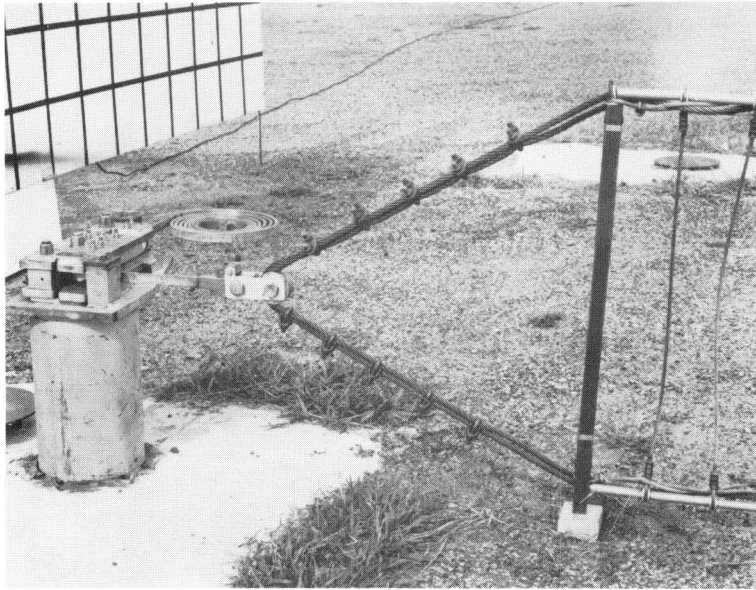
Figure 20, 12,500 Pound Metal Bender Before Test 505-4E. (Note smaller metal tape)
