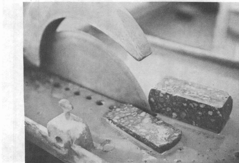
Fig. 2 Thin slabs 3\frac{1}{2} " x 1\frac{5}{8} " are sawed from the bituminous specimens. Slices from the top and bottom surfaces are used for testing.
