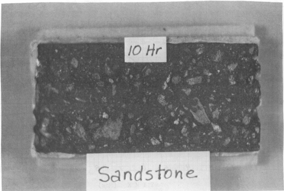
Fig. 9 Polish test coupon composed of sandstone aggregate from McMullen County shown at the completion of 10 hours of accelerated polishing. At the end of 13 hours, the polish value measured a 41. (Mag. 1.5X)
