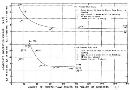
Freeze-Thaw Durability as a Function of AAF for Selected Synthetic Lightweight Concretes, by Code Number.
