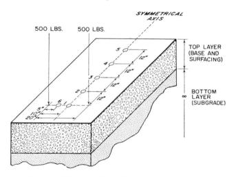
Relative position of Dynaflect loads and sensors. Vertical arrows represent load wheels. Points numbered 1 through 5 indicate location of sensors for standard test. Point 6 indicates the location of a desired additional measurement.
