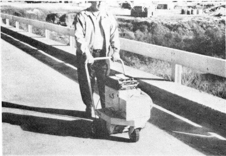
Delamination detector in operation.
