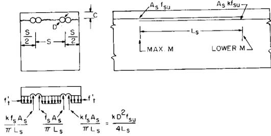
Fig. 4. Splitting forces for side split failure.
