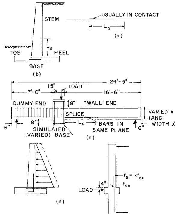
Fig. 1. Test concept. (b) Cantilever retaining wall with typical stem bar splices. (c) Test specimen to simulate wall splice. (d) Wall loading compared to test loading.
