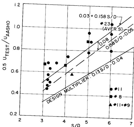
Fig. 3. Bond efficiency in terms of AASHO bond stress ( $0.75 \times 0.1f'_c \leq 0.75 \times 350$  psi).
