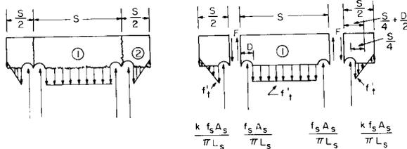
Fig. 5. Face-and-side split failure.
