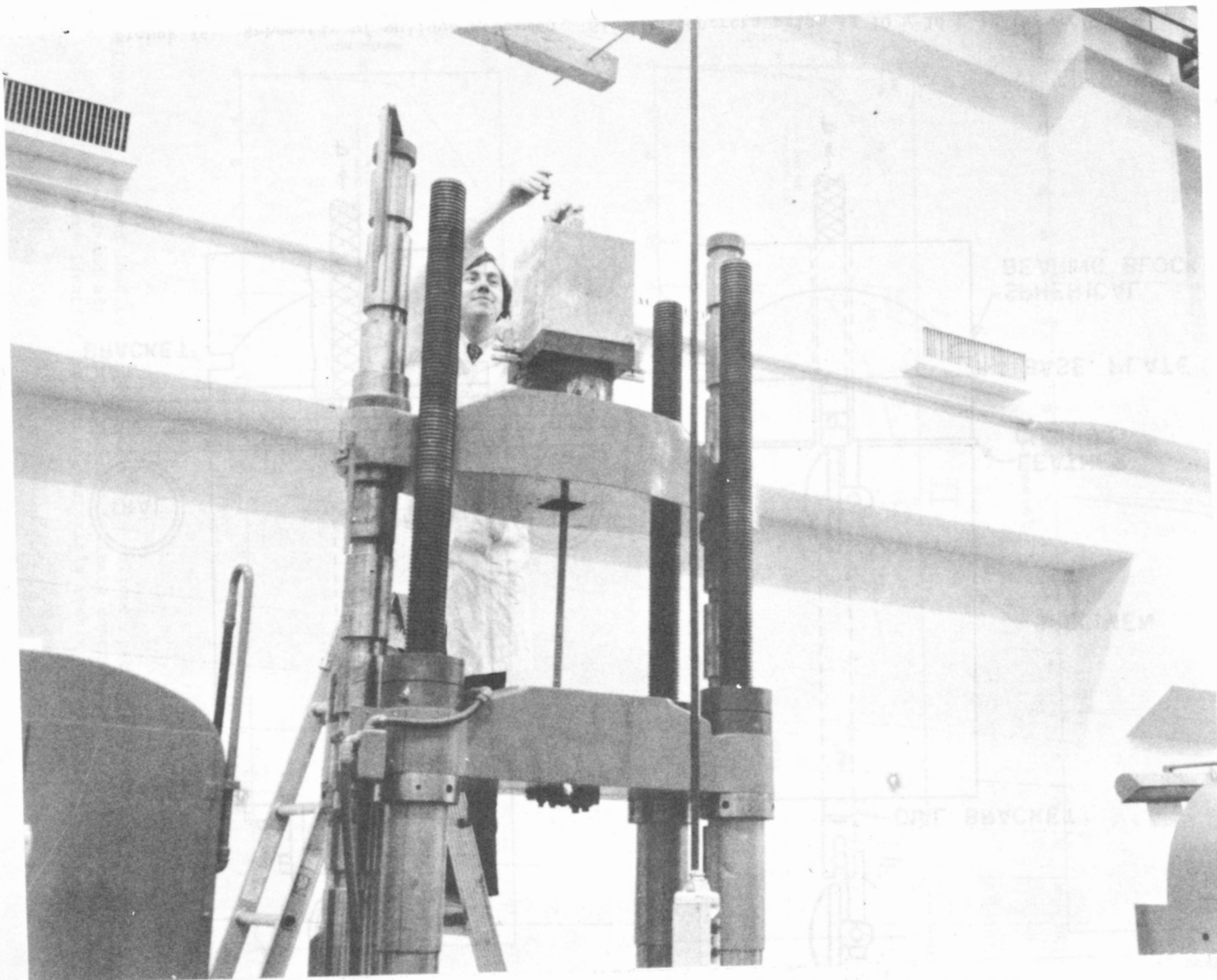
FIGURE 14. Pullout specimen on electromechanical testing machine being prepared for testing.
