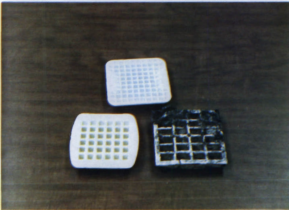
Figure 7: Various Waffle Bottom Markers. Note Epoxy did not fill the Waffle Bottom
