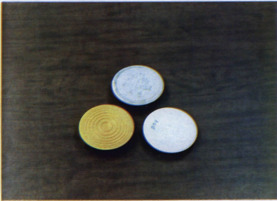
Figure 6: Showing the Plain and Concentric Rings on the Bottoms of Circular Markers
