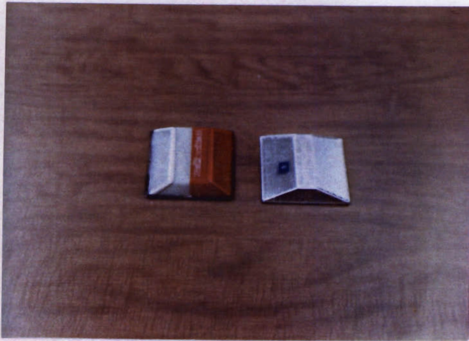
Figure 10: Stimsonite Reflective Marker. Right Marker has the 20° Incline. Left Marker has the 30° Incline
