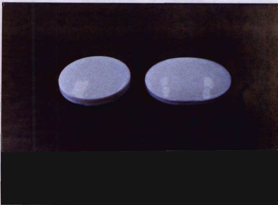
Figure 12: Showing Circular Dome Marker and the Original Oval Domed Flat Bottom Marker
