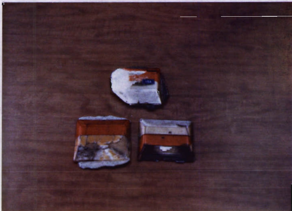
Figure 11: Typical Body Failures of Stimsonite Marker
