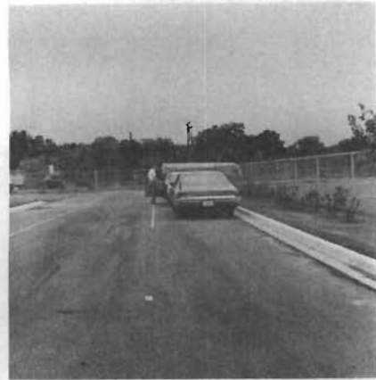
Figure 12. Encroachment of parallel parked vehicle and pedestrian on travel lane.
