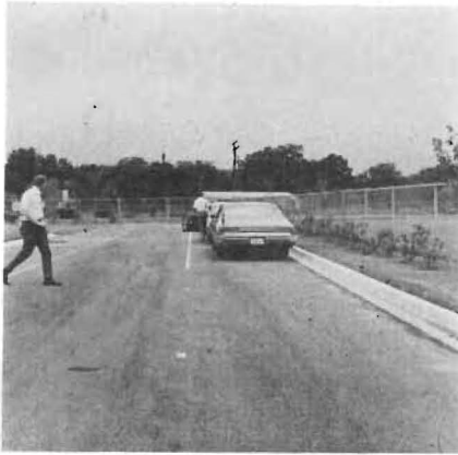
Figure 11. Encroachment of parallel parked vehicle and pedestrian on travel lane.
