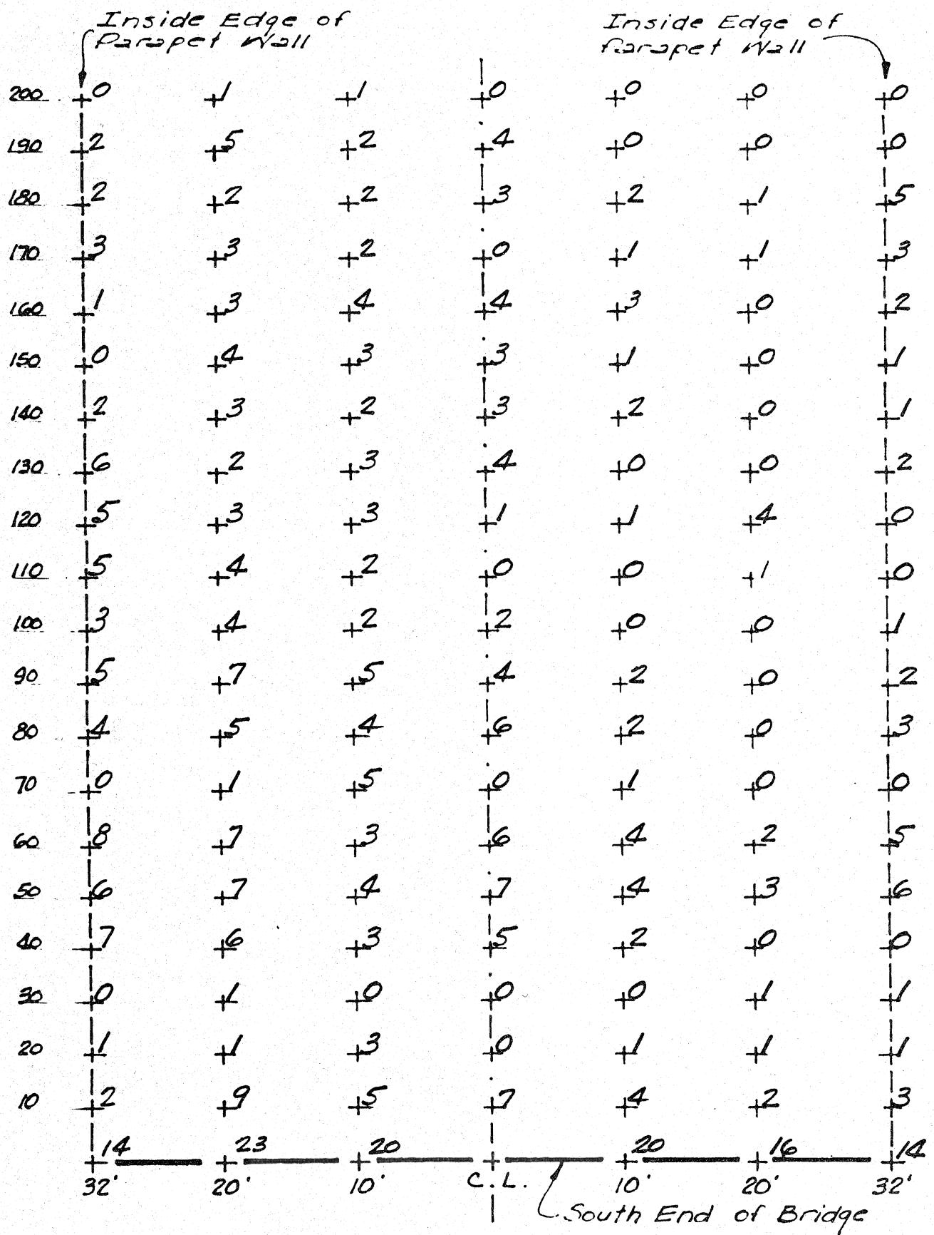
CORROSION POTENTIAL MEASUREMENTS
