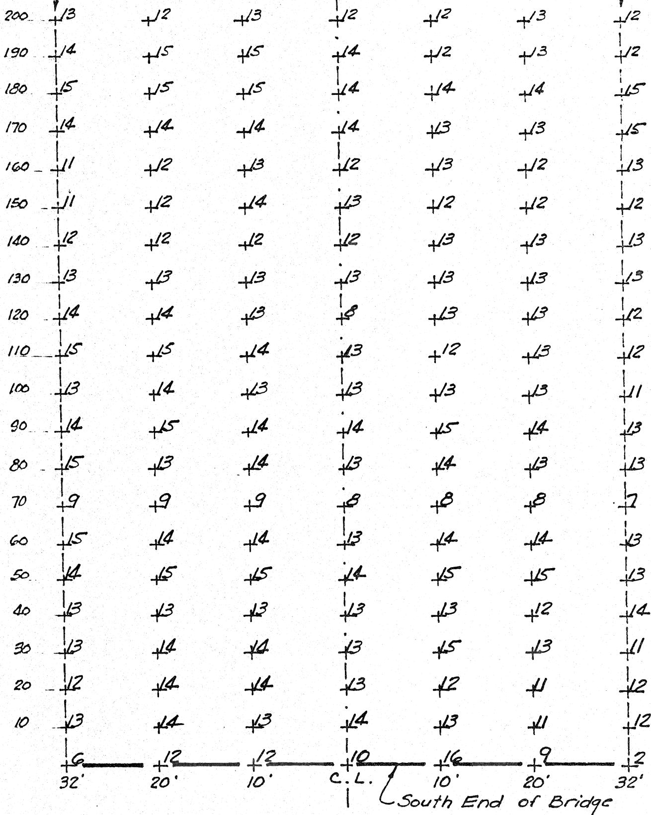
CORROSION POTENTIAL MEASUREMENTS
