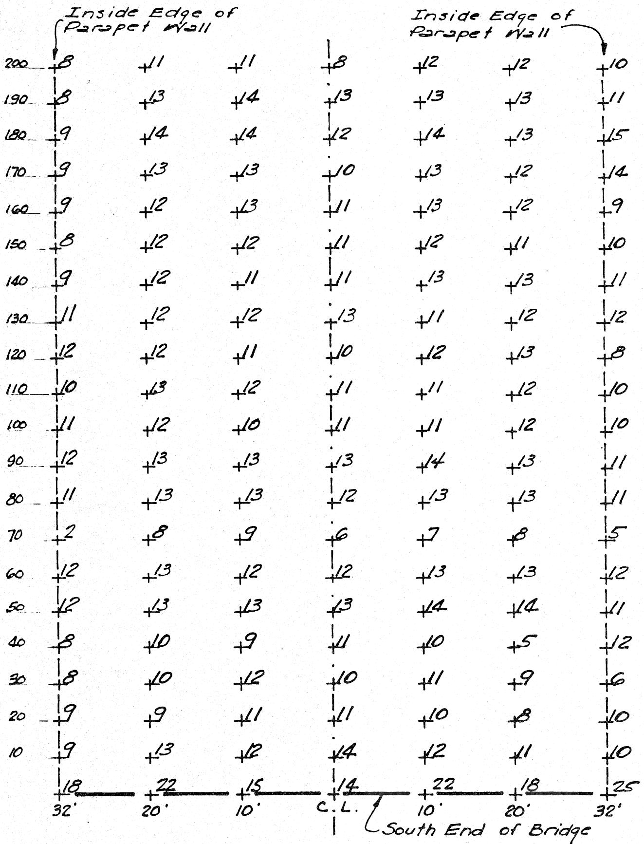
CORROSION POTENTIAL MEASUREMENTS
