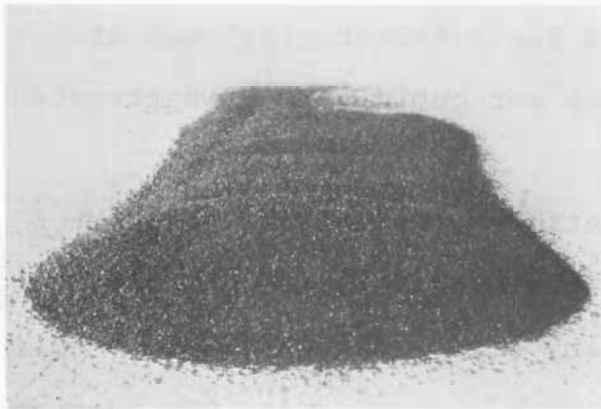
Plant Precoated Material Before Curing
