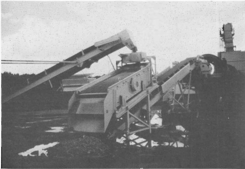
Figure 4.10. Scalping screen between gathering conveyor and incline conveyor (Ref 15).
