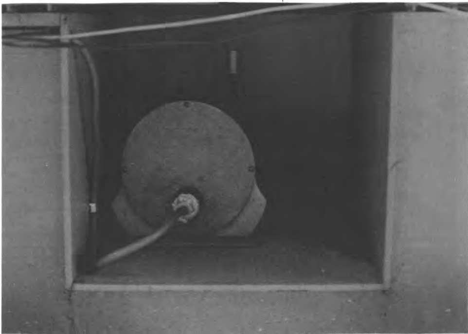
FIGURE 5 - TRAILER MOUNT OF MRM TRANSDUCER
