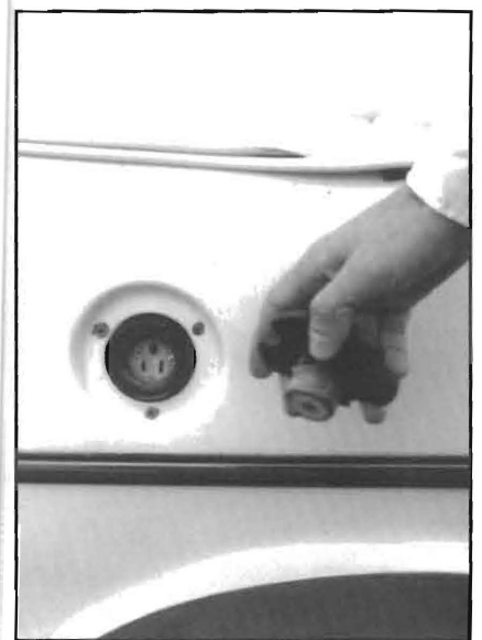
FIG. 6: The electric Rabbit is charged via a 110 VAC receptacle installed under the gas cap.
