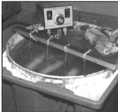
Fig. 1: Hot water immersion was one of several types of accelerated testing performed in 0-1265.
