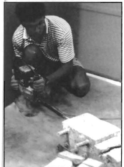
Fig. 2: Macro-cells had salt water ponded on top of them every other week. This set of cells was broken open after a year.
