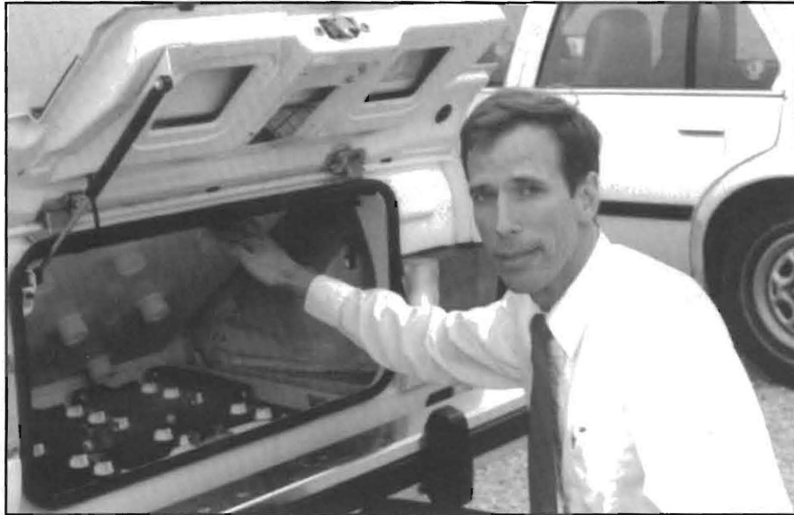
FIG. 5: Chris Harris reveals the aft eight of the sixteen 6-volt batteries powering the Rabbit. The batteries are enclosed in a polypropylene box.
