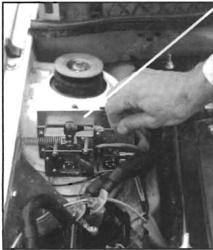
FIG. 3: The throttle potbox is simply attached to the vehicle's original throttle cable and pedal. It sends a variable resistance signal to the speed controller to specify the amount of electricity to be released to the motor.
