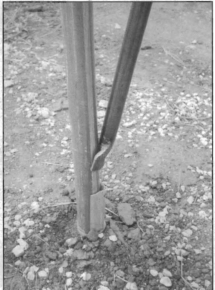
FIG. 3: The wedge driver head fits securely against the post.
