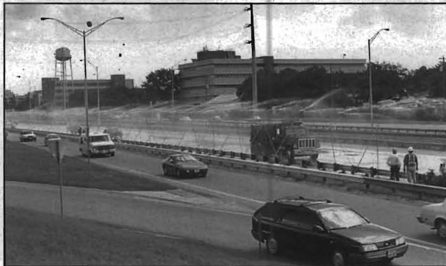
FIGURE 1: The rain simulator in action on MoPac.
