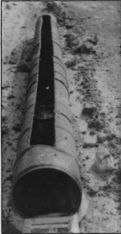
FIGURE 2: The flush tank, made from 16-gallon barrels, has hook grabs on each end for lifting off and on the trailer.
