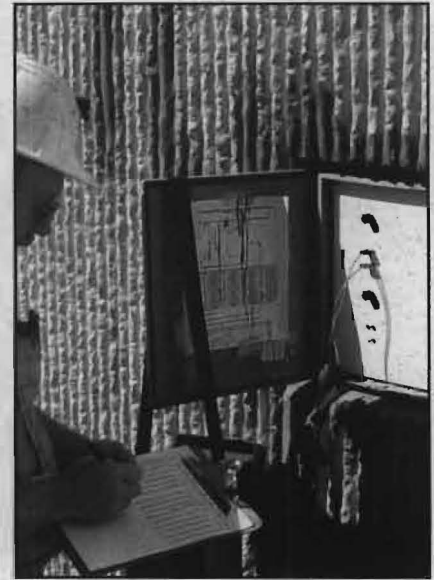
FIG. 4: Gathering strain gauge and other data for performance evaluation.
