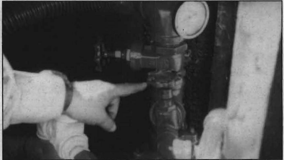
FIGURE 3: Discharge valve (red) — sends material back into distributor or emulsion tank.
