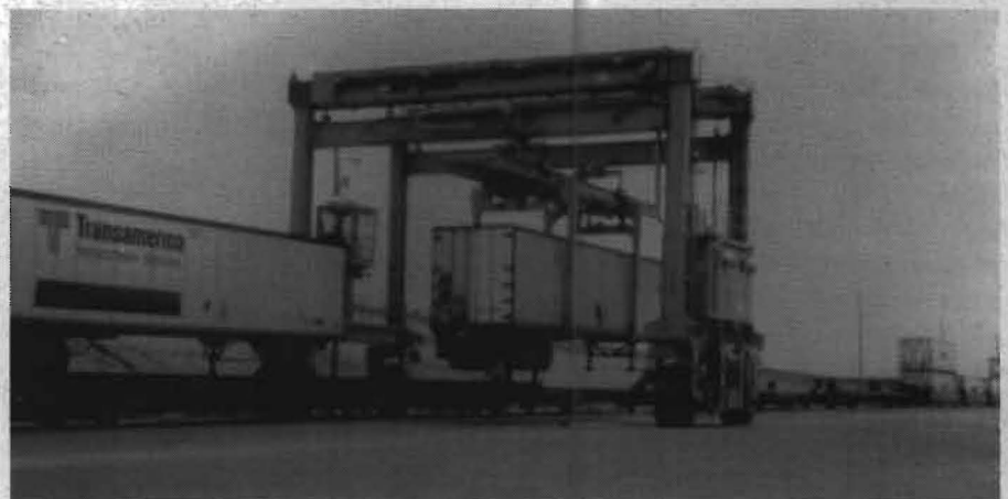
FIGURE 5: An intermodal yard crane lifts a semitrailer onto a flatcar.
