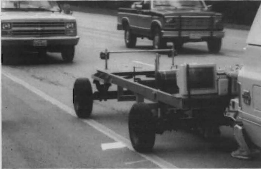
FIGURE 1: SHRP prototype seismic pavement analyser built at UTEP detects very early pavement damage for preventive maintenance.
