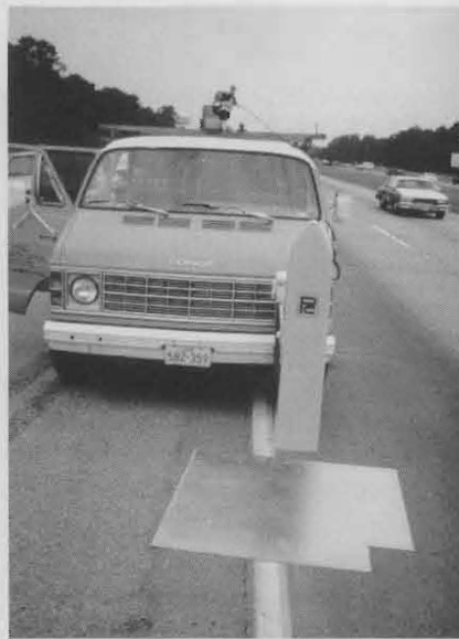
FIGURE 1: The GPR system.
