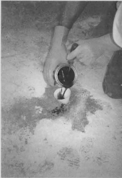
FIGURE 4: Filling dry-drilled hole with red epoxy.
