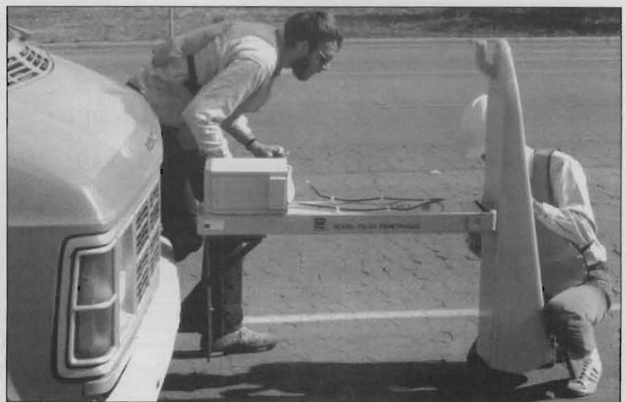
FIGURE 4: Truck-mounted ground penetrating radar.
