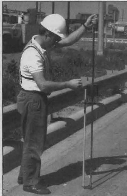
FIG. 3: Dynamic cone penetrometer.
