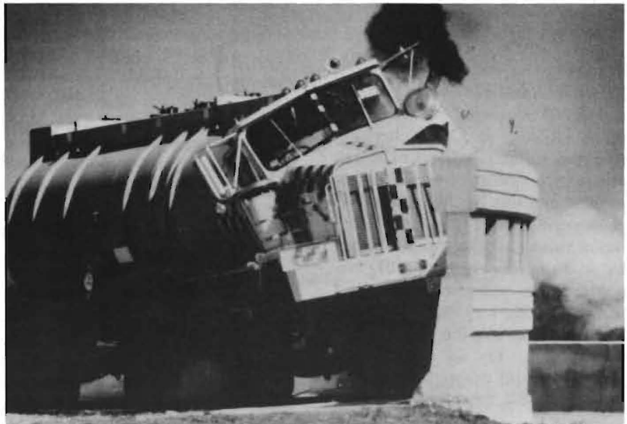
FIGURE 1: A possible application for stronger-than-average concrete: Bridge rails to contain and redirect 80,000 lbs trucks.
