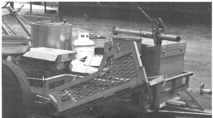
FIGURE 6 Hinged platform folded, seat stowed, applicator secured by winch.
