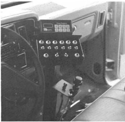
FIGURE 5 Digital display and spray pump throttle.
