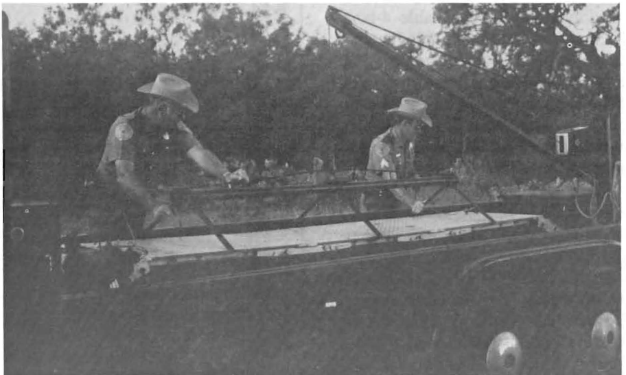
FIGURE 5 The semi-portable ramped axle-group [AX/GRP (RAM)] scale.
