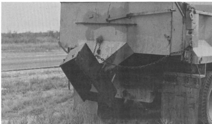
FIGURE 1 The modified box and tailgate arrangement.
