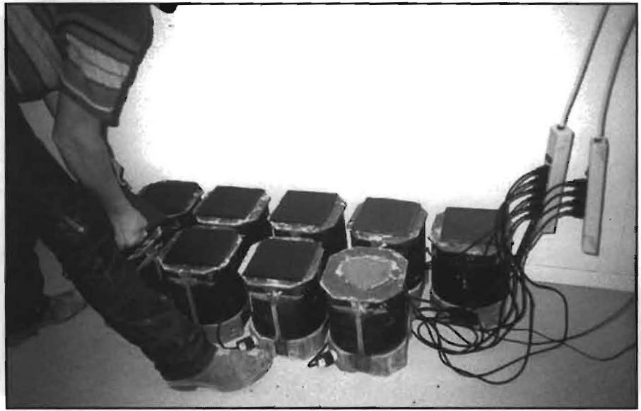
FIG. 7: Match-cured cylinder mold system.
