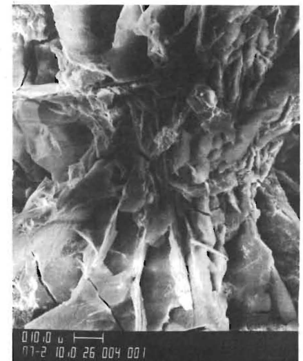
FIGURE 6 Boxwork rust crystals growing within portland cement concrete.
