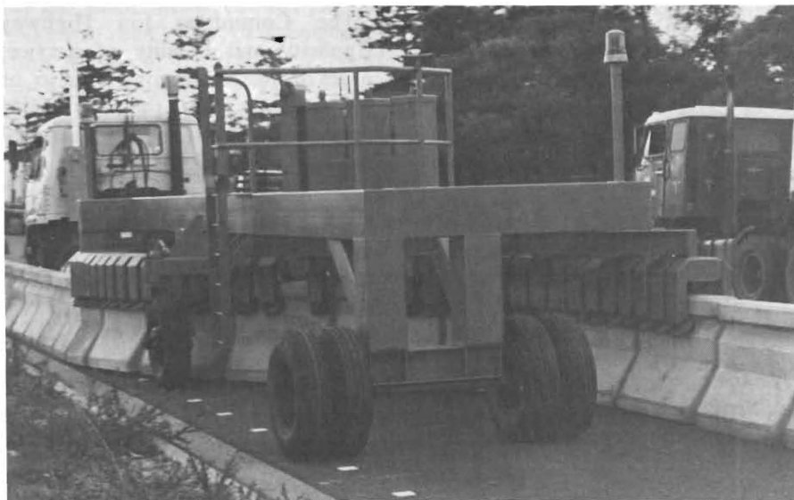
FIGURE 1 The towed transfer unit.
