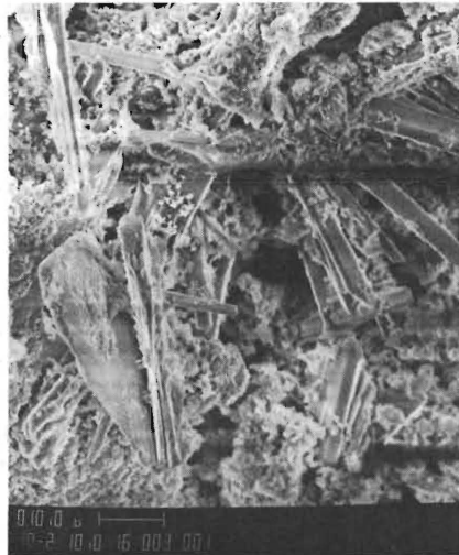
B, Rust crystals found 2 inches from corroding reinforcing steel.
