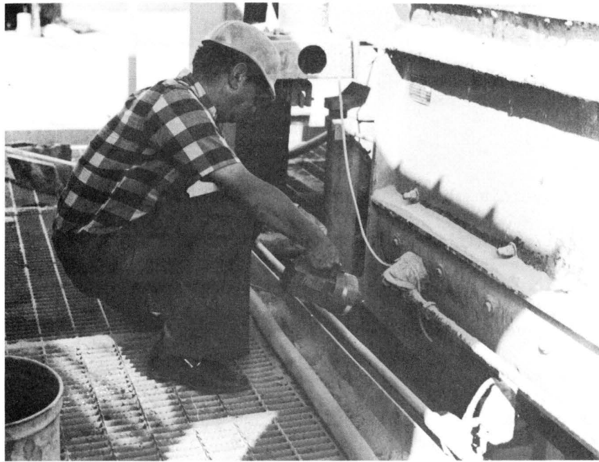
Figure 26. Monitoring H 2 S emissions with a Metronics "Rotorod" gas sampler.
