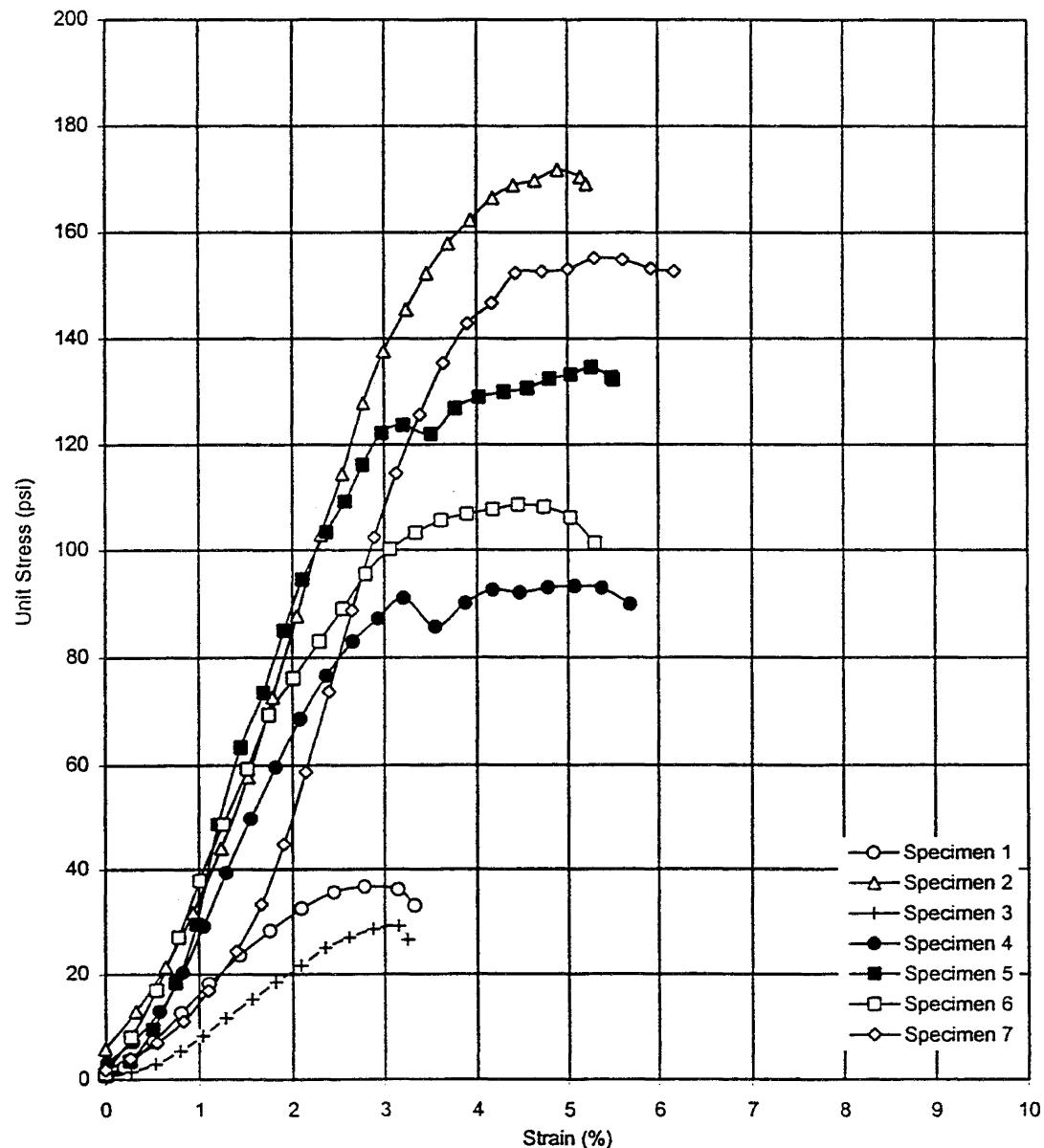
**Note:** A compressive stress was recorded at zero strain due to (1) weight of porous stone & bell housing, and (2) compressive stress induced by applying lateral pressure while restraining the specimen to read zero strain prior to shearing the specimen.
