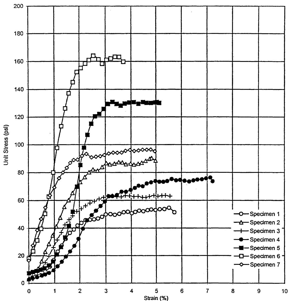
Note: A compressive stress was recorded at zero strain due to (1) weight of porous stone & bell housing, and (2) compressive stress induced by applying lateral pressure while restraining the specimen to read zero strain prior to shearing the specimen.
