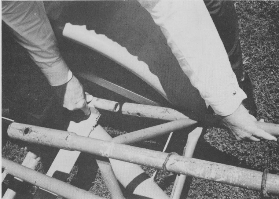
Figure 9 : Back end of front section of profilometer mast is supported by rod inserted into mast leg. Other leg rests on trailer tongue.
