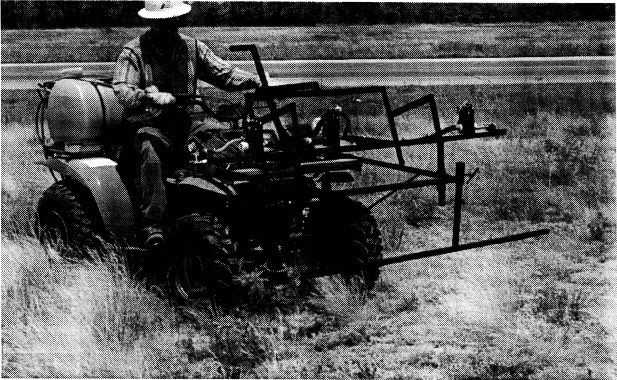
Figure 6. First prototype of an automatic ATV sprayer with 3 nozzles for selective application of leaf sprays to mesquite across a 2.74-m-wide swath.
