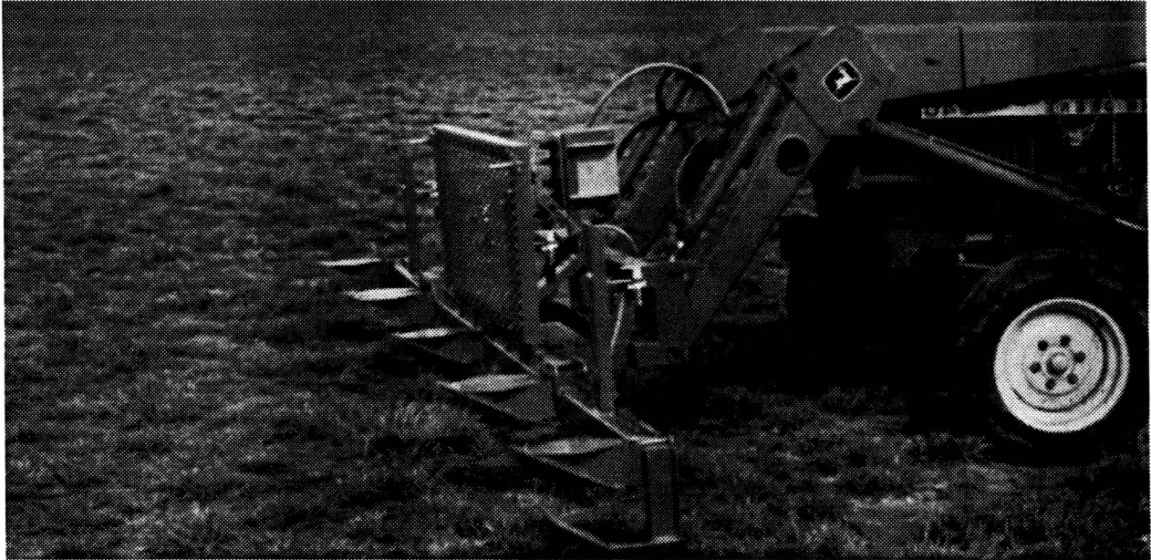
Figure 7. First prototype of the 3.66-m mesquite-sensing spray boom, which automatically and selectively applies leaf sprays to mesquite after their leaves or stems break horizontal beams of modulated light.
