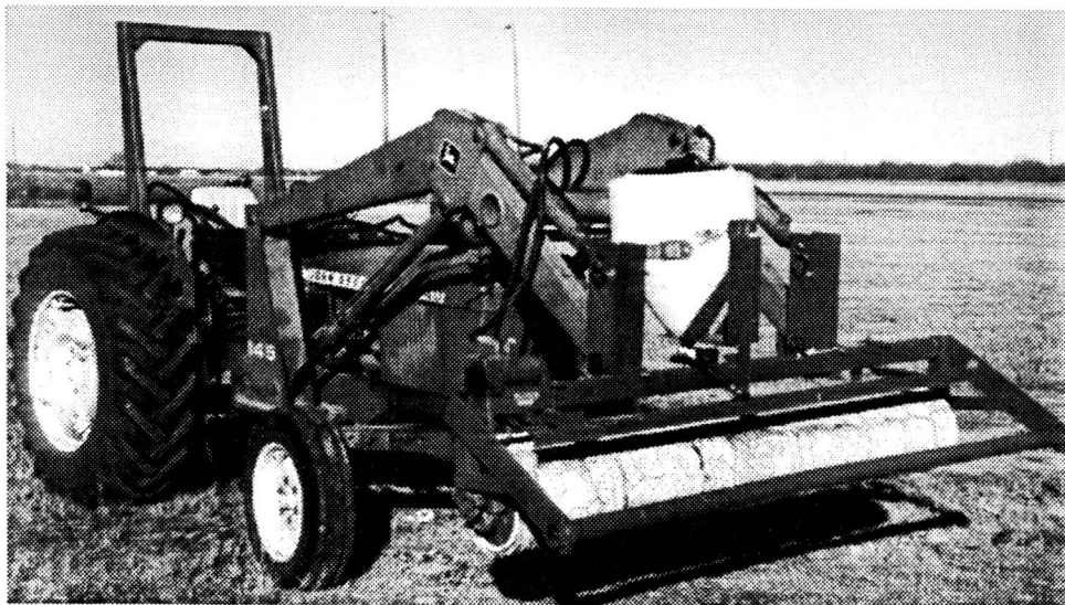
Figure 4. Carpeted roller with 1.98-m wide, carpet-covered, rotating cylinder for selective application of herbicide solution to mesquite in highway rights-of-way.
