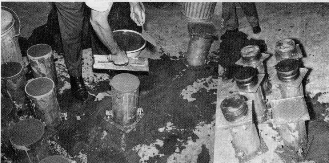
Fig 8. Capping operation on 6 x 12-inch specimens.
