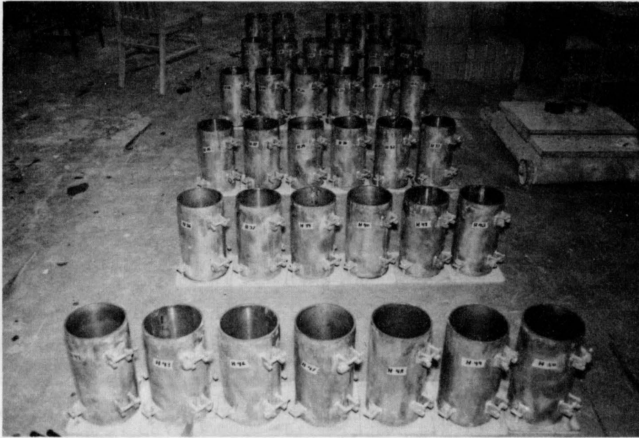
Fig 5. The 6 x 12-inch molds ready for casting. Copper inserts in some molds are for as-cast specimens.
