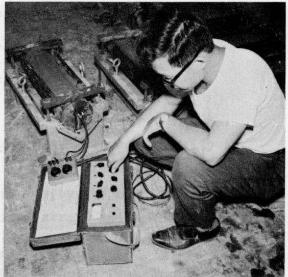
b. Comparator used with specimens immediately after casting.
