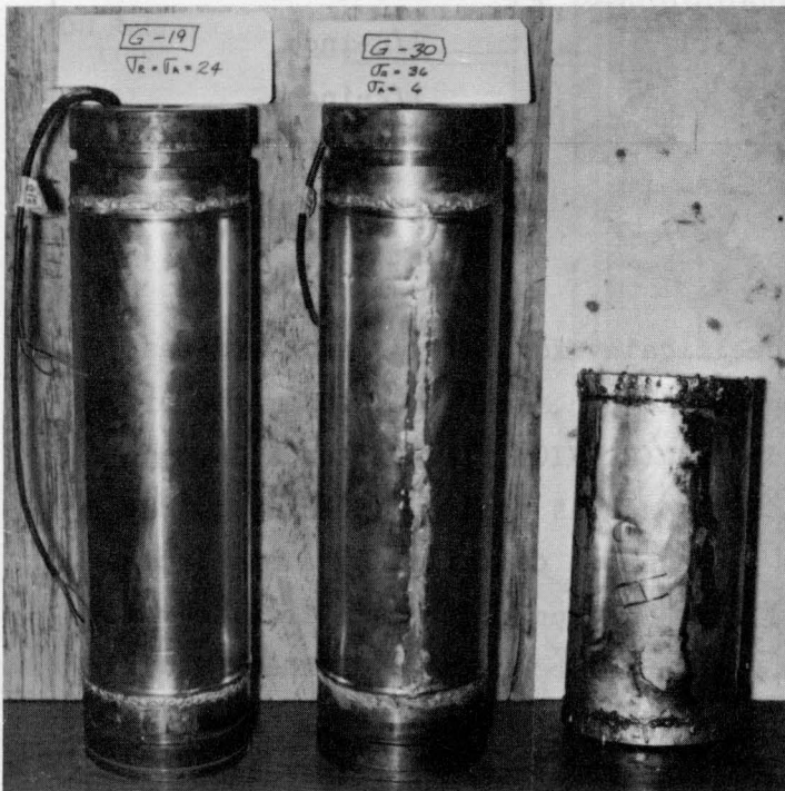
c. 6 x 12-inch concrete specimens after completion of soldering copper jackets.
