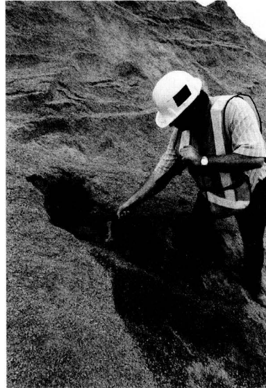
TxDOT inspectors collect materials samples from the materials stockpile locations.
