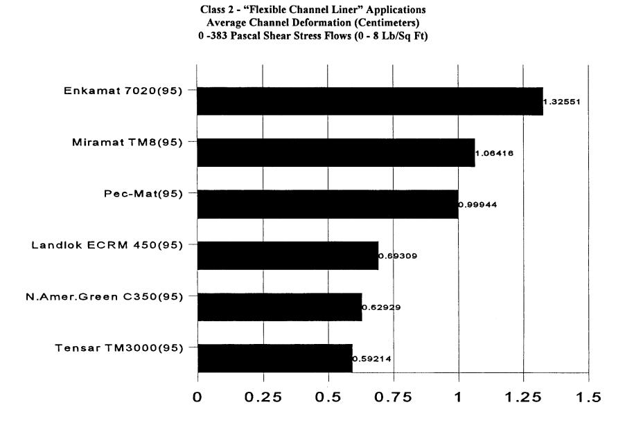
1995 Evaluation Cycle TxDOT/TTI Hydraulics and Erosion Control Laboratory Class 2 "Flexible Channel Liner" Applications
