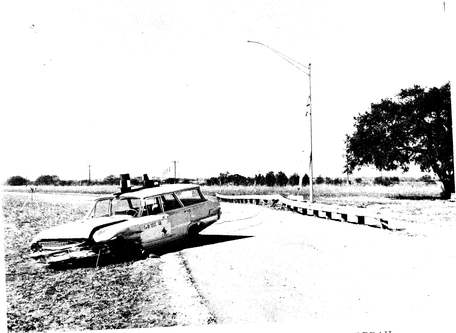
FIGURE A.6 DAMAGE TO TEST VEHICLE AND GUARDRAIL
