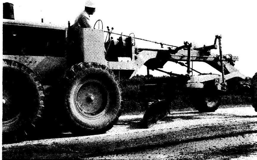
ANGLE-BLADE POSITION TO SPREAD MATERIAL TO RIGHT
