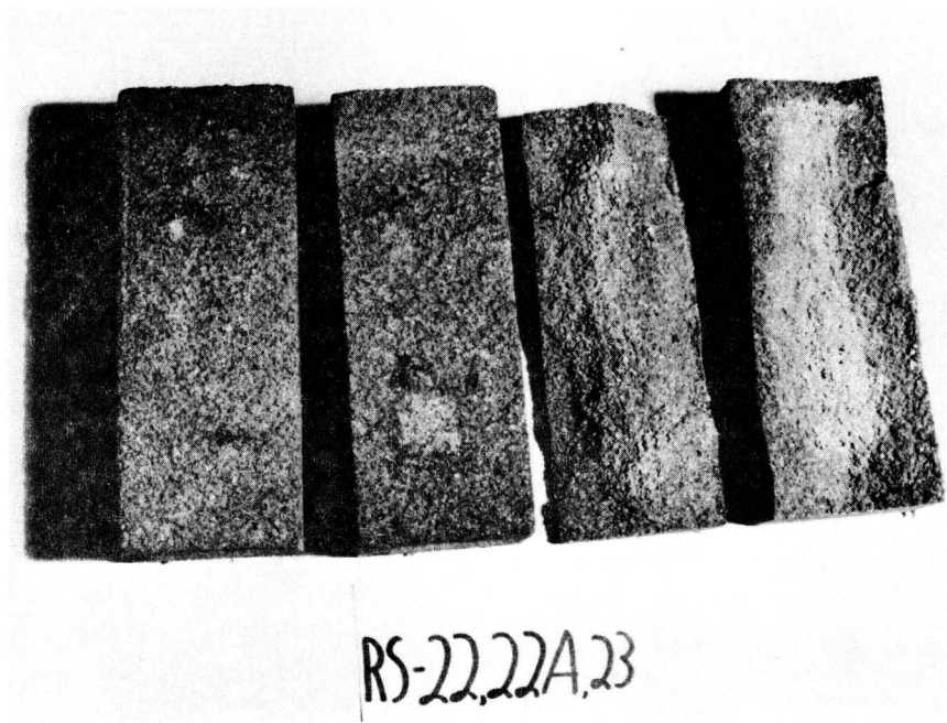
Figure C7 Conditions of specimens RS-22, 22A after 27 cycles, and RS-23 after 4 cycles of freezing and thawing.
