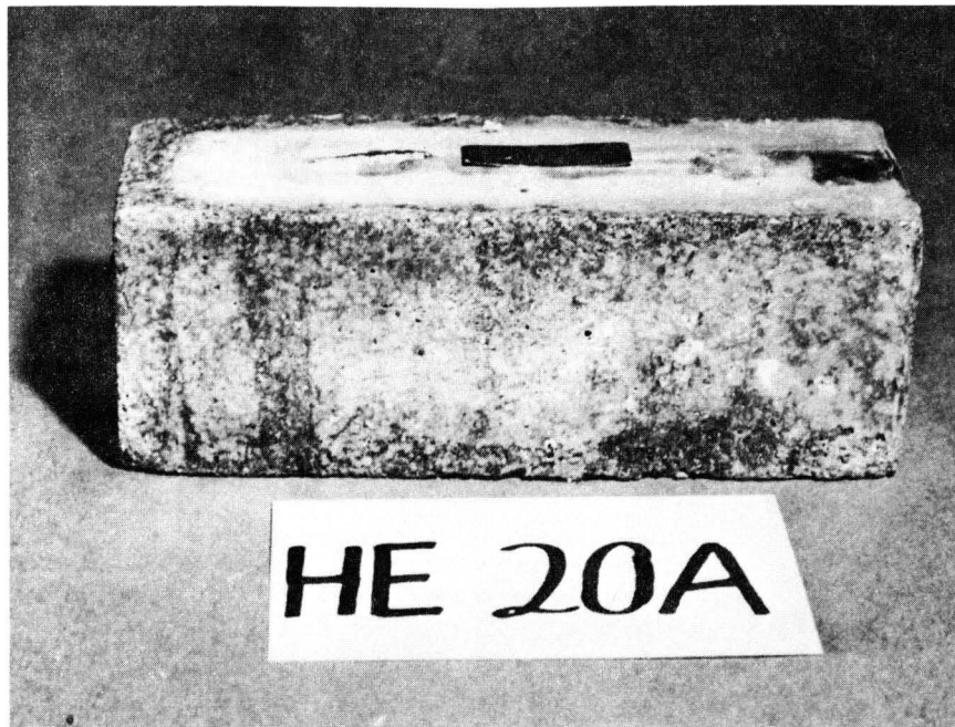
Figure C15 Condition of specimen HE1-20A after 16 cycles of freezing and thawing.
