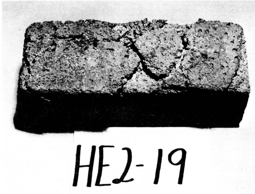
Figure C18 Condition of specimen HE2-19 after 23 cycles of freezing and thawing.
