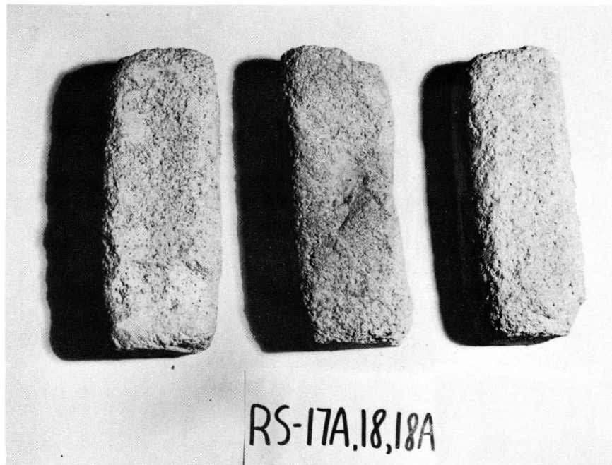
Figure C2 Conditions of specimens RS-17A, 18, 18A after 11 cycles of freezing and thawing.
