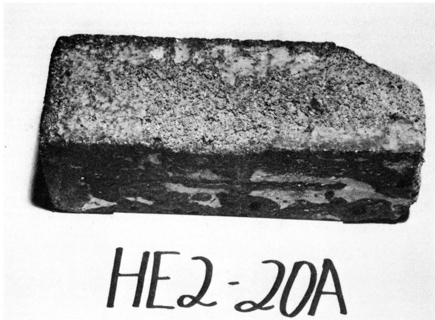
Figure C21 Condition of specimen HE2-20A after 36 cycles of freezing and thawing.
