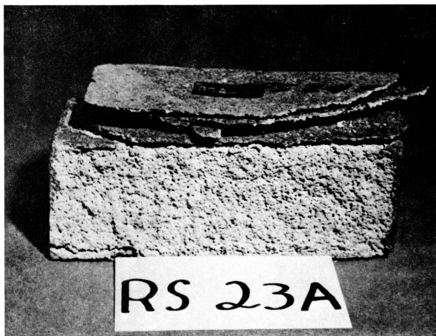
Figure C8 Condition of specimen RS-23A after 19 cycles of freezing and thawing.
