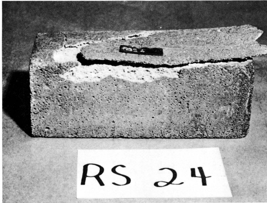
Figure C9 Condition of specimen RS-24 after 14 cycles of freezing and thawing.
