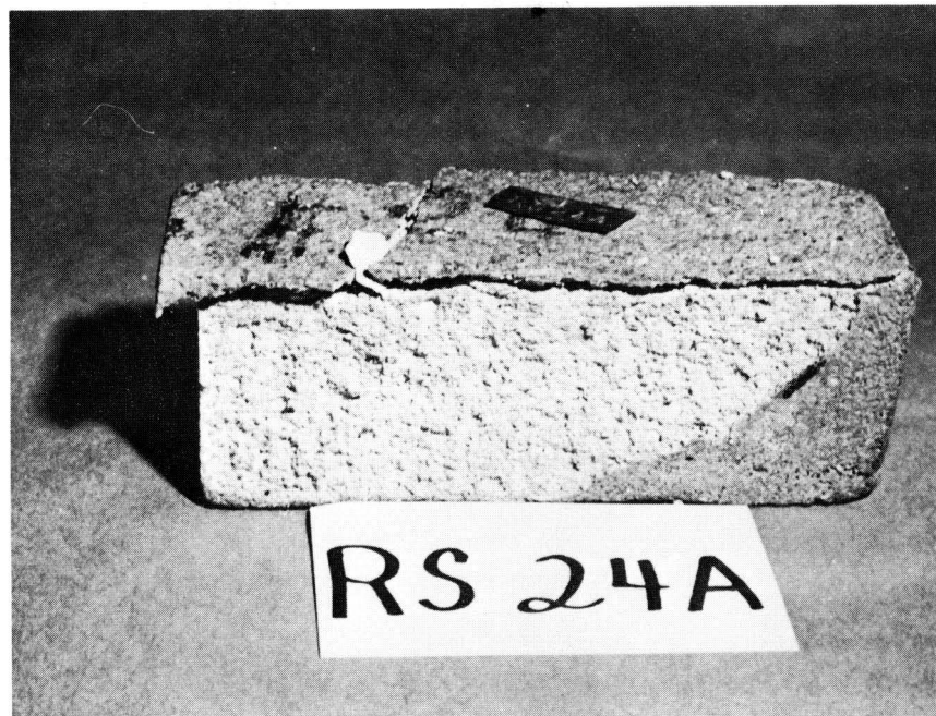
Figure C10 Condition of specimen RS-24A after 16 cycles of freezing and thawing.
