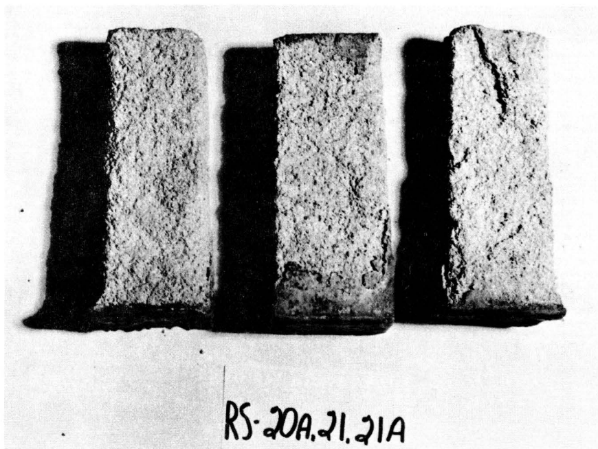
Figure C4 Conditions of specimens RS-20A, 21, 21A after eight cycles of freezing and thawing.
