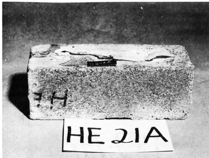
Figure C17 Condition of specimen HE1-21A after 16 cycles of freezing and thawing.
