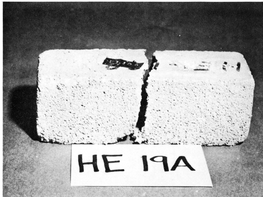
Figure C13 Condition of specimen HE1-19A after 24 cycles of freezing and thawing.
