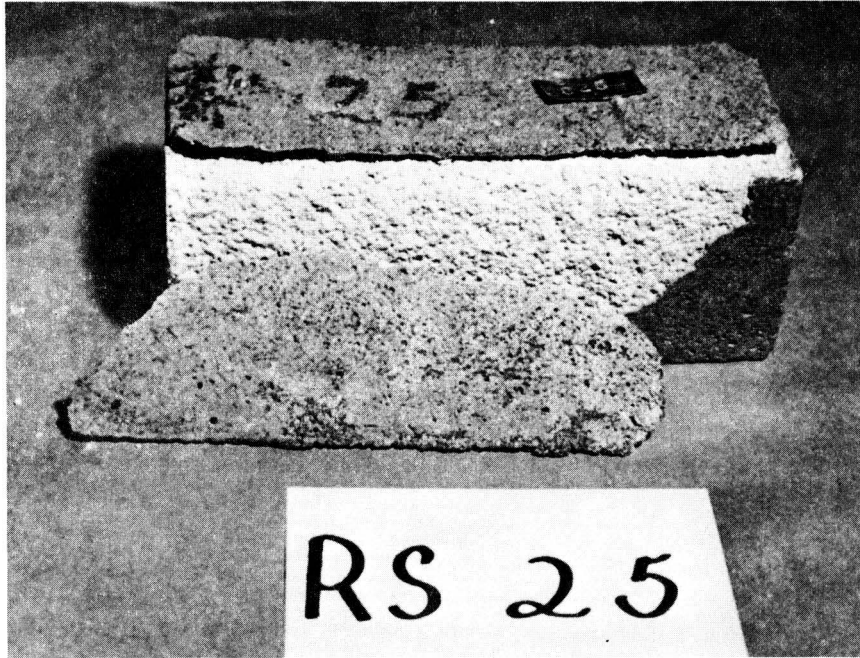
Figure C11 Condition of specimen RS-25 after 8 cycles of freezing and thawing.
