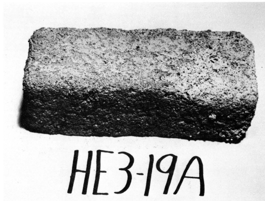
Figure C25 Condition of specimen HE3-19A after 37 cycles of freezing and thawing.
