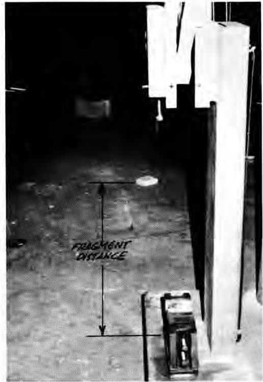
Figure 4: AFTER IMPACT, DISTANCE TO FRAGMENT WAS MEASURED
