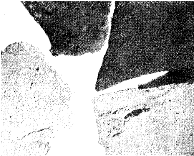
Figure 2. Particles of TXI-Eastland. (Mag. 7-1/2X)
