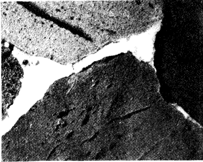
Figure 1. Particles of TXI-Eastland material showing internal bloating features. (Mag. 7-1/2X)
