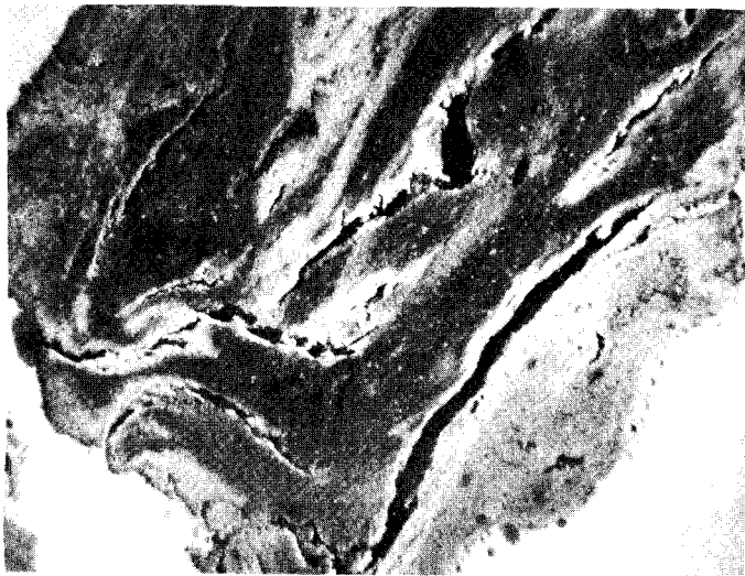
Figure 3. Particle showing cracks along the contorted bedding planes. The external color is orange and the interior is gray. (Mag. 7X)
