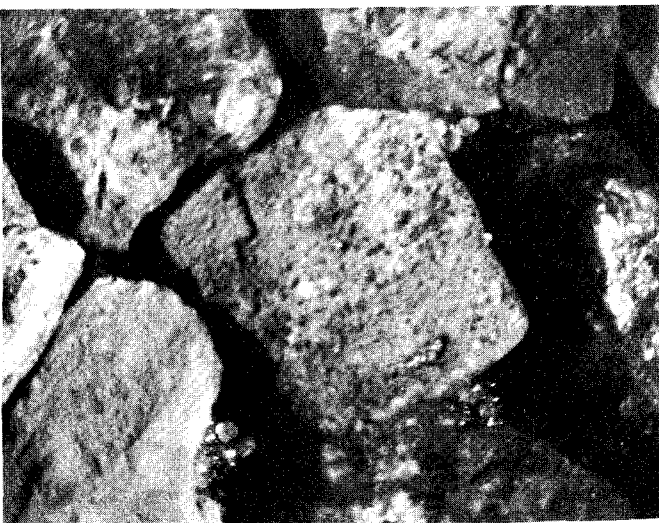
Figure 3. View of polish value sample showing abraded particles of TXI-Eastland material. (Mag. 3X)
