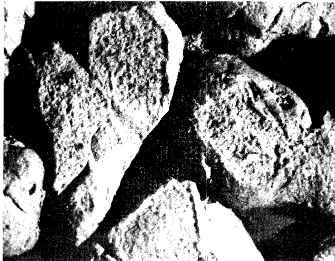
Figure 5. Same as above. Note more resistant rind in relief after the polish test. (Mag. 7X)
