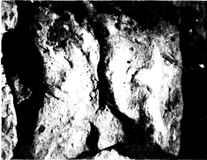
Figure 5. Particle showing microtexture resulting from sand inclusions in addition to crack systems. (Mag. 7X)
