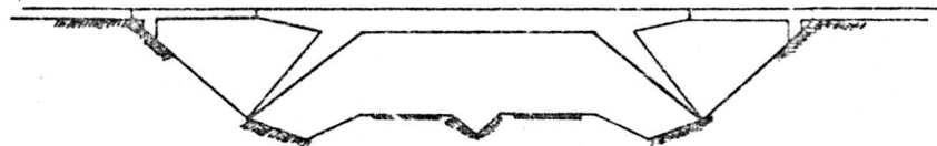
FIGURE 6. PRESTRESSED (POST TENSIONED) CONCRETE BRIDGE CONCEPT
