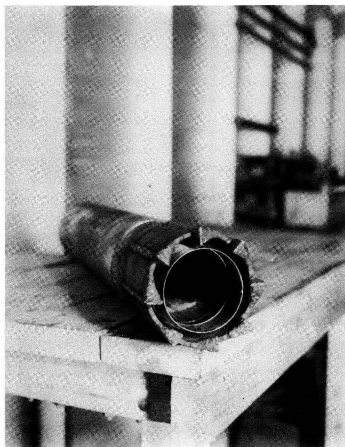
FIG. 2-B WET BARREL SAMPLER
