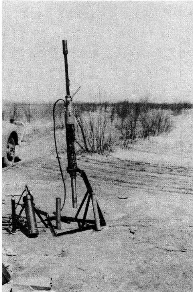
FIG. 2-E. COHESIONLESS SAND SAMPLER
