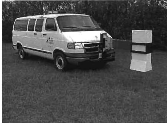
Figure 2.8 - Photograph of GPR
