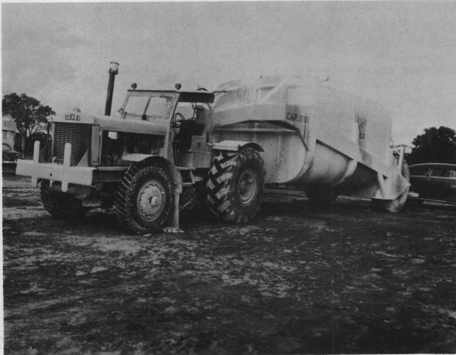
Photograph No. 30 Contractor adapts Euclid earth moving equipment into slurry tank in the Bryan District.
