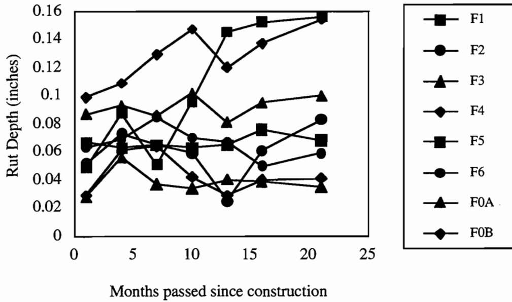
Figure 6.13 Rut depth versus time at inside wheel path in right lane — Flexible section
