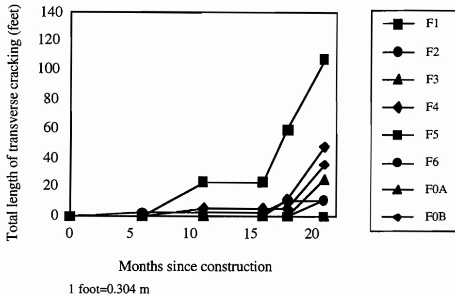
Figure 7.19 Total length of transverse cracking in left lane
