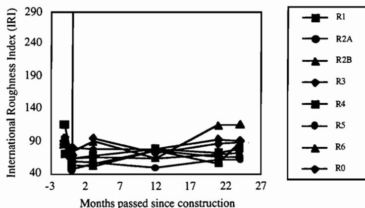
Figure 8.12 IRI versus time at outside wheel path of left lane — Rigid section
