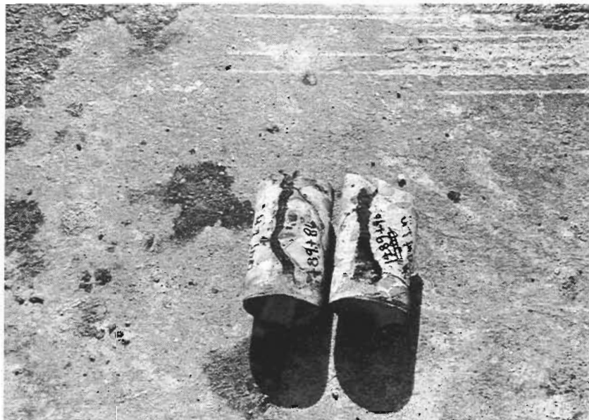
Figure 3.7. Cores taken from Monomer repair
