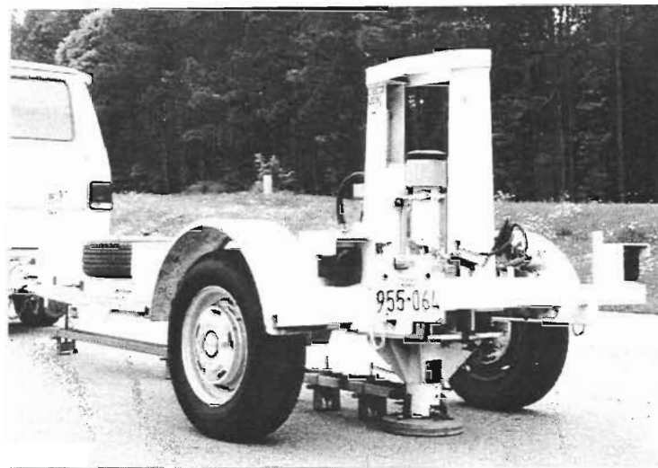
Figure 2.1. The FWD operating within the flexible sections
