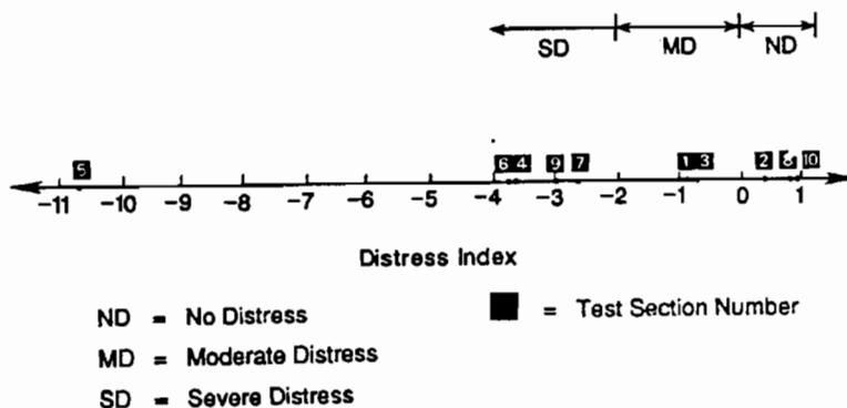
Fig 2.1. A line diagram of distress index of each test section.
