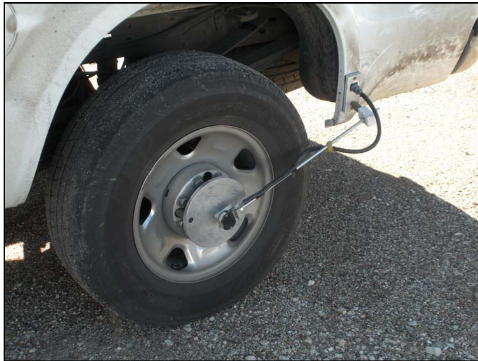
Figure 5. Distance Measuring Assembly Used on TTI Profiler.
