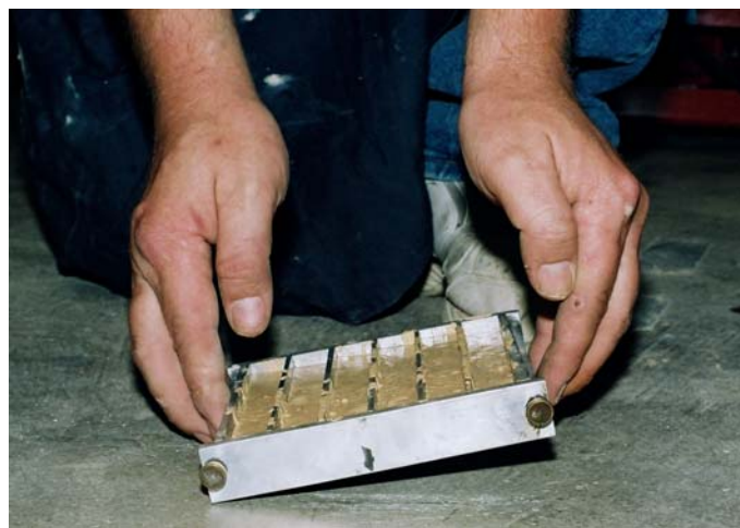
Figure 3.4 Sample Consolidation by Lifting One Side of the Tray and Dropping it on Hard Surface
