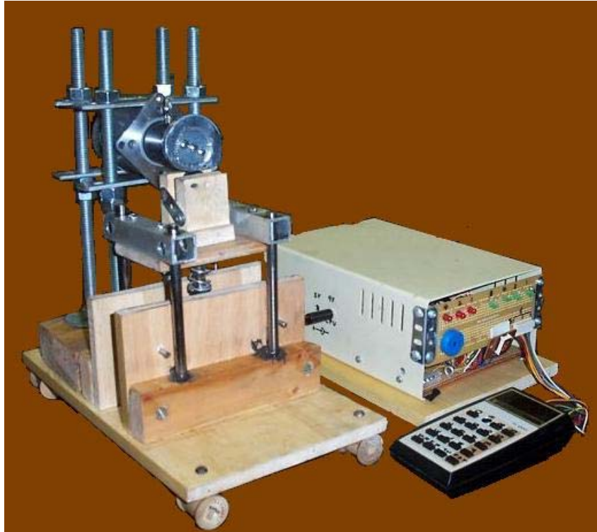
Figure 3.8 Loading Device with Cam and Spring Mechanism
