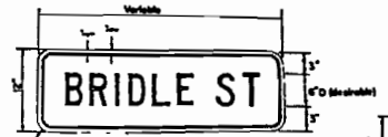
M4-9N Letters - Black Border - Black Background - Orange Reflective The M4-9R, L or S sign is to be used to detour local streets or roads that are not a State or Federal numbered highway; however, it should not be used in lieu of the M4-10 sign at the beginning of the detour or to detour State or Federal numbered routes.
