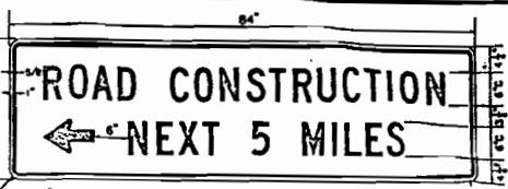
G20-1bL G20-1bR 84" x 24" Letters - Black Numerals - Black Border - Black Background - Orange Reflective Arrow - Black
