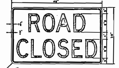
R11-2 48" x 30" STREET [ ] 6" R11-2S RAMP [ ] 6" R11-2R Letters - Black Border - Black Background - White Reflective
